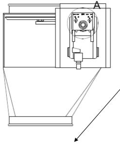
\*Release button for sealed door - shall be released when cleaning. **REMEMBER to turn off the power!!!**
